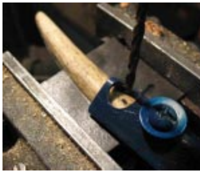
Figure 6: Drill jigs in use
