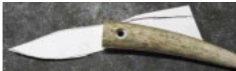
Figure 12: Paper blade in place
